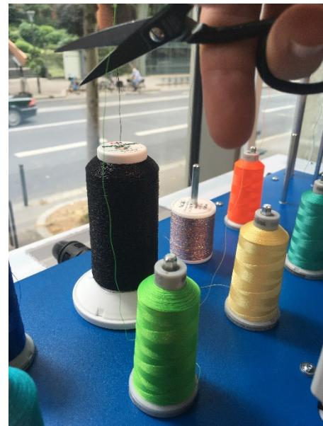
**SELECT** the needle location to be used (here needle #10) and **LOCATE** the corresponding installed spool (the green thread spool).
