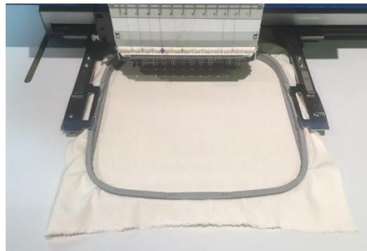
*Frame correctly installed.*
