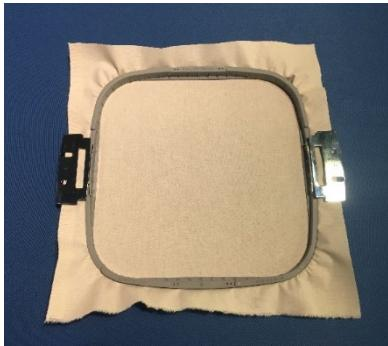
**PLACE** the "ear" frame on top. Push until the upper frame is pushed into the lower frame.
