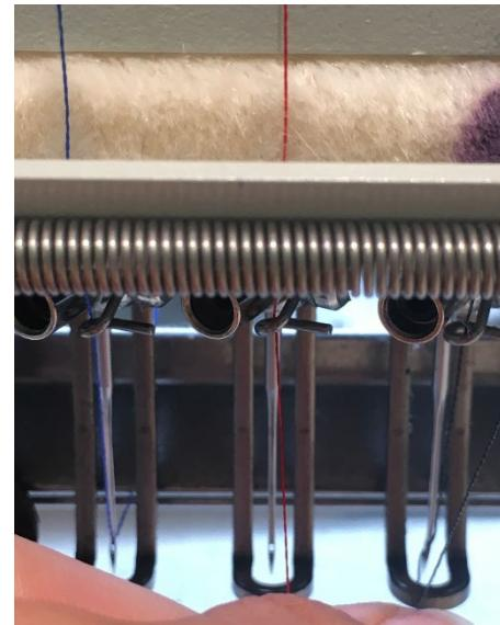
**PASS** the red thread through the metal loop at the top of the needle.
