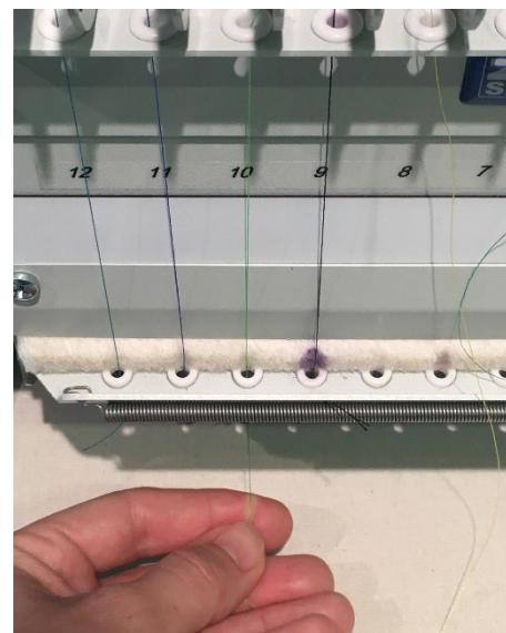
**PULL** the thread already in place by taking it out of the eye of the needle
