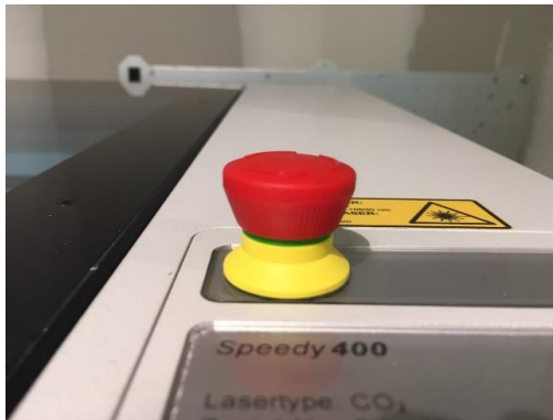
Emergency stop button armed > I see the green ring = you can use the machine
